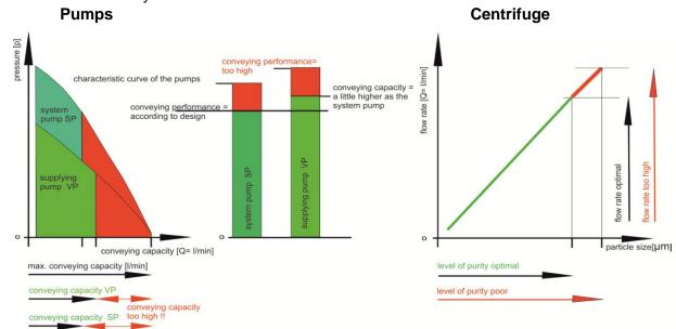
Adjust system pump SP according to the design of the unit. Conveying capacity is depending on the pressure. Operating point inside the green area!
