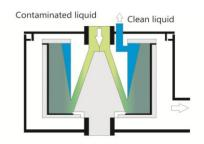
The centrifuge separates solids from liquids using centrifugal forces.
